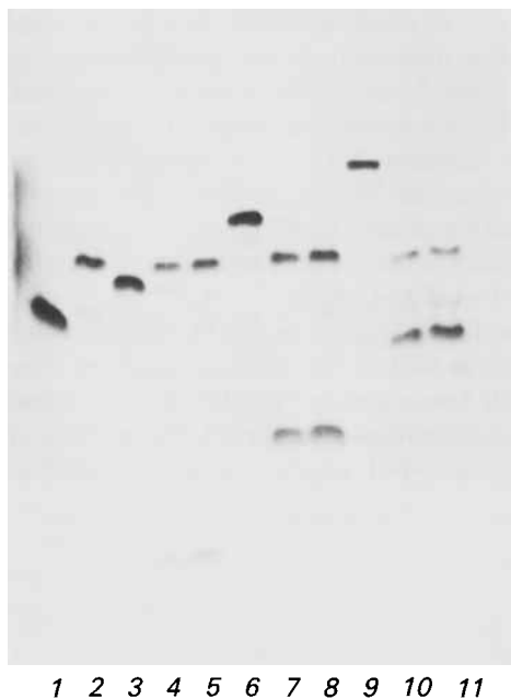
Fig. 1. UV-Shadowing gel electrophoresis of the products in the stepwise synthesis of 11 and cleavage products thereof. Lane 1: crude 7 ; lane 2: crude 8 ; lane 3: crude 9 ; lane 6: crude 10 ; lane 9: crude 11 ; lanes 4, 5: cleavage of crude 9 with 80% AcOH after 2 and 6 h; lanes 7, 8: cleavage of crude 10 with 80% AcOH after 2 and 6 h; lanes 10, 11: cleavage of crude 11 with 80% AcOH after 2 and 6 h.
